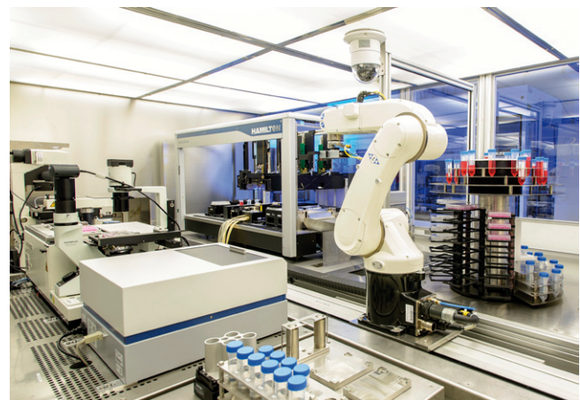
Fig. 4: StemCellFactory, an automatic production facility for patient-specific iPS cells.
