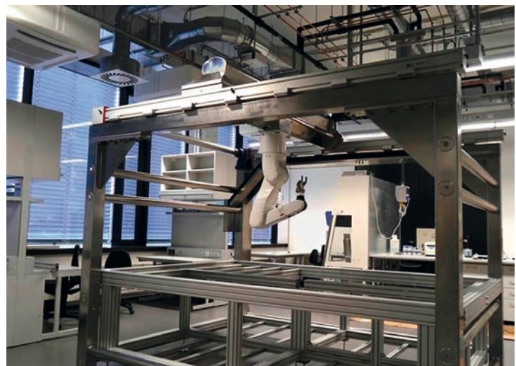
Fig. 3: New robotic system for automatic iPS cell production under construction.
